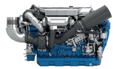
Number of cylinders Bore and stroke Total displacement Engine rotation Idle speed Flywheel housing Flywheel 6 127 x 165 mm 12.5 L Counterclockwise 700rpm SAE 1 SAE 14"
