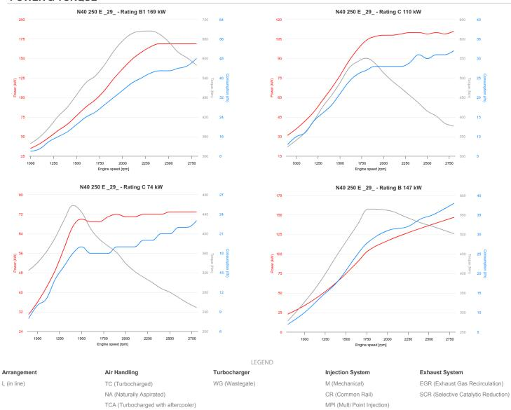
A1 High Performance Crafts. Full throttle operation restricted within 10% of total use period. Cruising speed at engine rpm <90% of rated speed setting - Maximum usage 300 hours per year.
